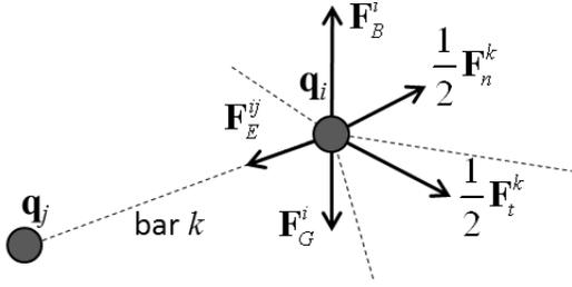
Fig. 5. The force distribution for a mass point  $i$ .
