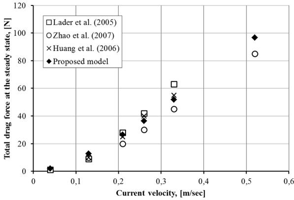
Fig. 8. The comparison of the total drag force with other research works (Huang et al. [7], Lader et al. [12], Zhao et al. [6]).
