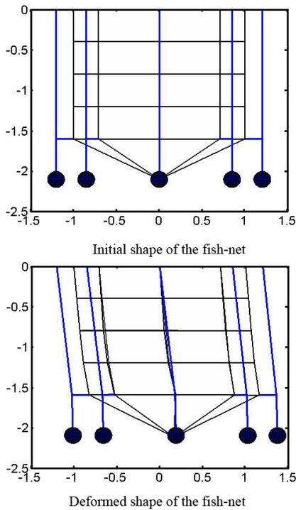
Fig. 9. Simulation results of the full aquaculture fish-net structure.
