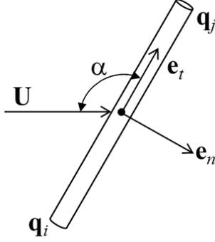
Fig. 3. Normal and tangential unit vectors and angle of attack definitions.
