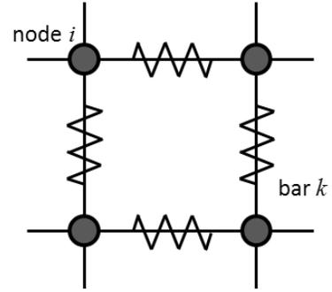
Fig. 2. A schematic diagram of a lumped-mass model.
