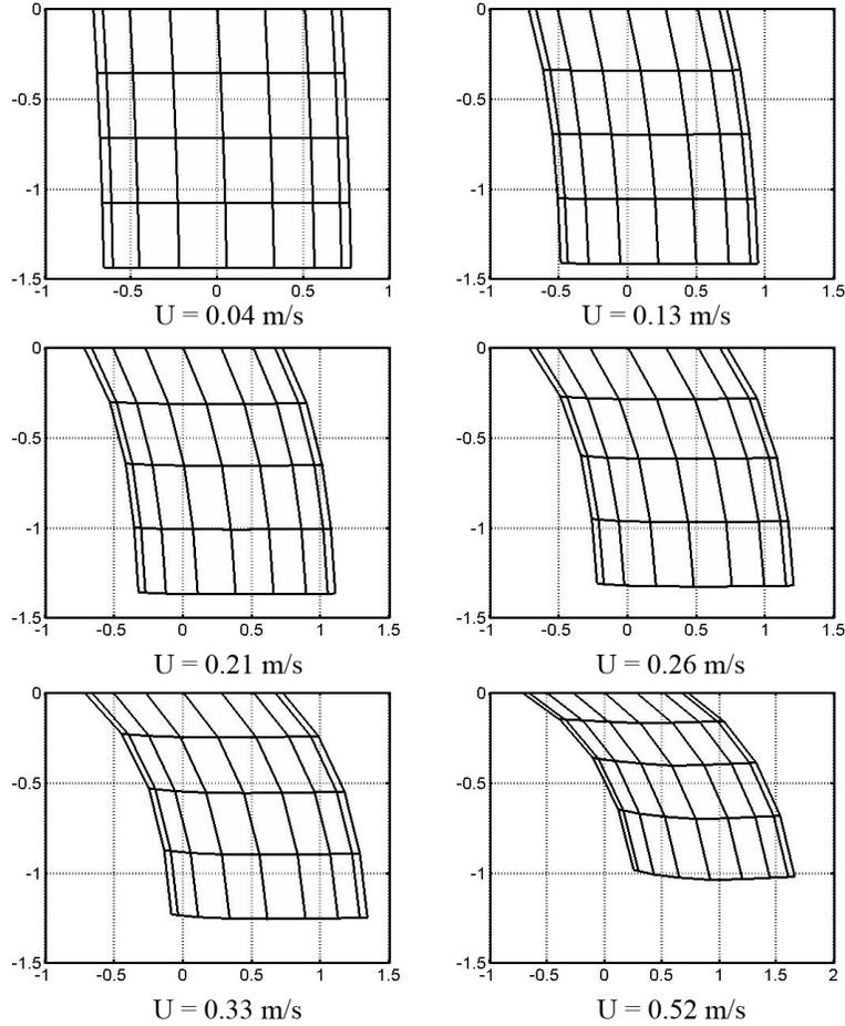
Fig. 7. Simulation results of the fish net structure for different current velocities.
