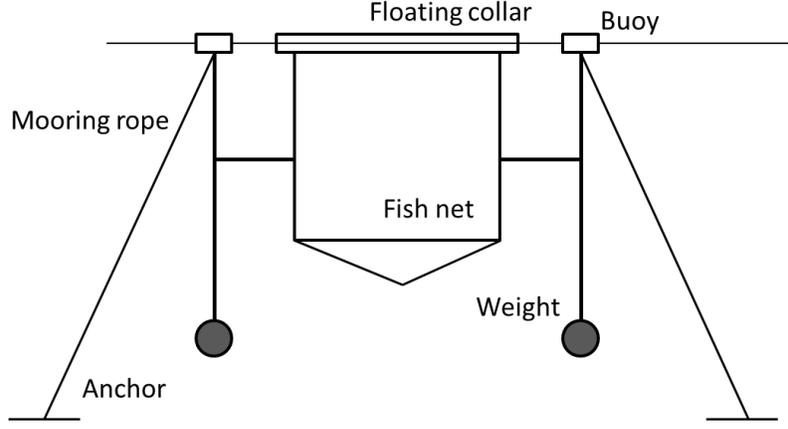
Fig. 1. An example of a fish cage system.
