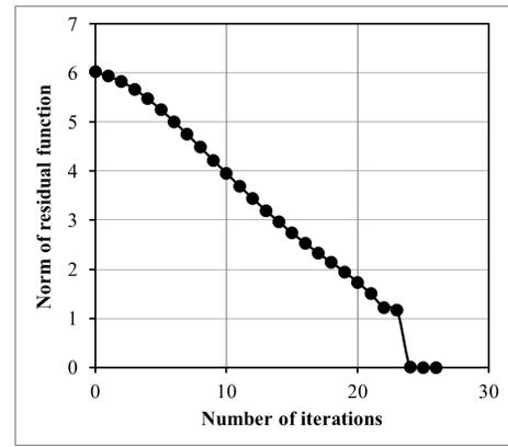
Fig. 10. The residual norm as a function of the iteration number for the current velocity updating.
