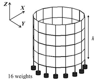
Fig. 6. A net model used in simulations.
