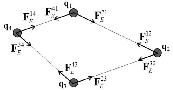
Fig. 4. The structural forces of mesh bar elements.
